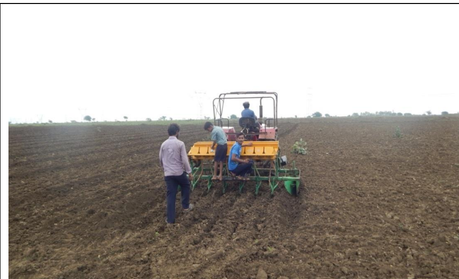
Assessment of Broad bed planter for broad bed method of soybean cultivation
