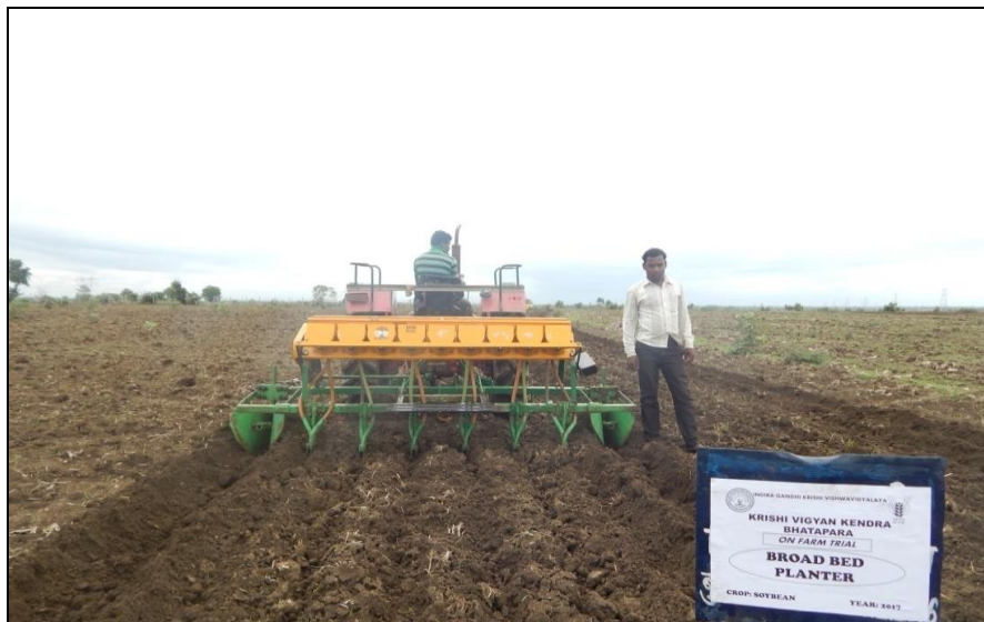
Assessment of Broad bed planter for broad bed method of soybean cultivation
